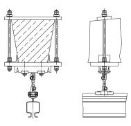
Embracing brackets clamp around the building trusses so that drilling completely through them is not necessary.
